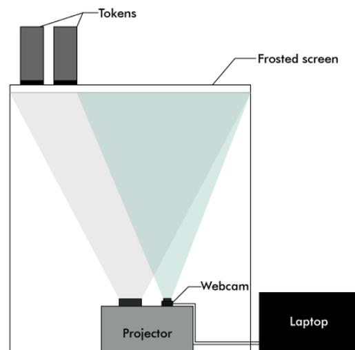
**Figure 2: System's equipment schematic arrangement**
